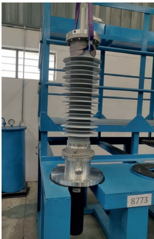
◀ Assembled 75.5 kV bushing on a technological rack
