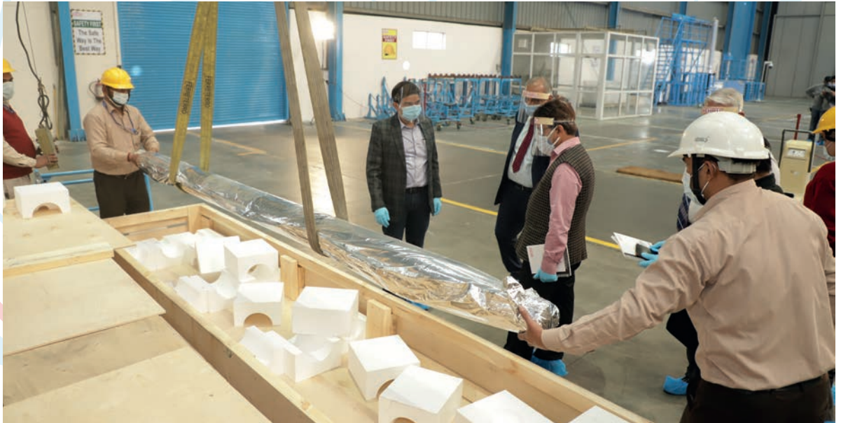
▼ A 145 kV insulation core with preinstalled mounting flange is all ready for final assembly
