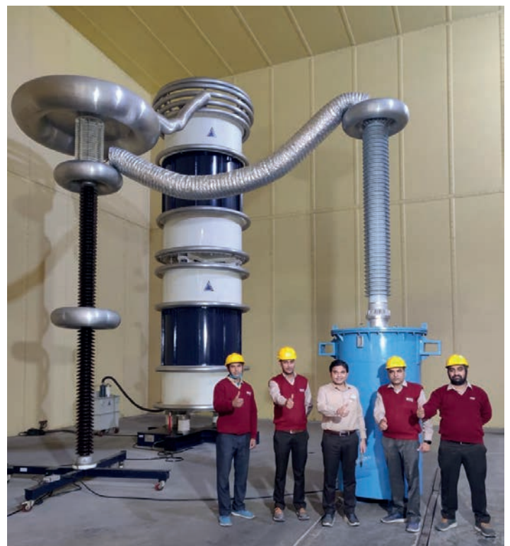
◀ Assembled 75.5 kV bushing on a technological rack
