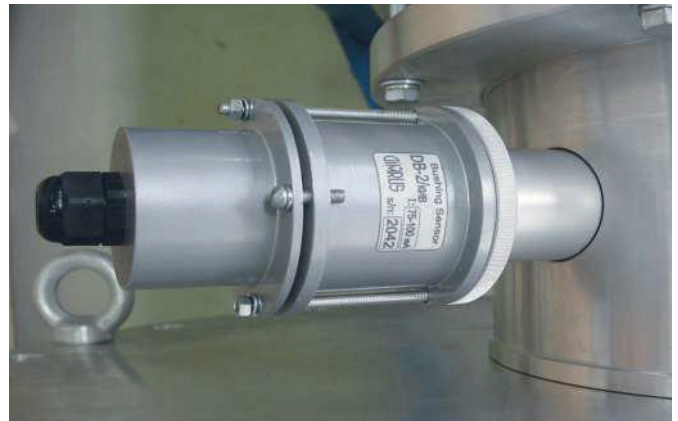
Fig. 7. Sensor for protection of the test tap
